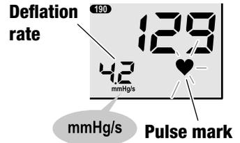
When measurement ends, air is rapidly exhausted, and then the measurement result is displayed.
