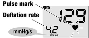
When measurement ends, air is quickly exhausted, and then a countdown (15 seconds) starts.
